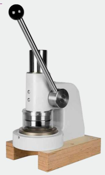
The robust round sample punch is mounted on a heavy, bonded plywood base. The round blade is forced through the die with a hand lever and the sample is expelled downwards. An acrylic glass safety guard surrounds the upper blade.
